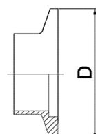
**Application:** Vacuum systems that function in a rough, fine and high vacuum, (10–9 mbar depending on the seals), for positive pressure applications up to 2.5 bar
