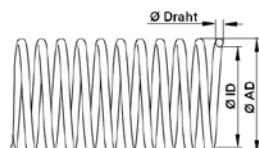
Round spring steel wire protective helix protects the hose against extreme external abrasion.
